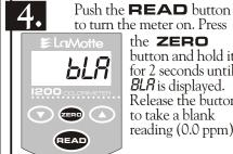
the ZERO button and hold it for 2 seconds until **BLR** is displayed. Release the button to take a blank reading (0.0 ppm).
