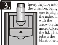
the chamber, being sure to align the index line with the arrow on the meter. Close the lid. This tube is the blank or zero.
