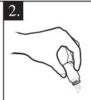
Rinse and fill a colorimeter tube (0290) to the 10 mL line with sample water. Cap and wipe dry.
