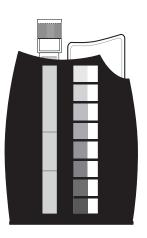
The Octa-Slide 2 Viewer should be held so non-direct light enters through the back of the Viewer. Insert the reacted sample into the top of the Viewer. Slide the Octa-Slide 2 Bar into the Viewer and match the color of the reaction to the color standards.
